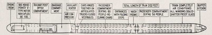
car body forms a deep stiff beam, thereby requiring a minimum amount of material for a given strength.
