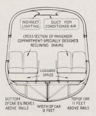
The train is fully air conditioned; windows sealed, and forced ventilation used which will heat the train in winter, cool it in summer, filter all dirt and dust from the outside air and maintaining a pressure in the car, will exclude all dirt.
