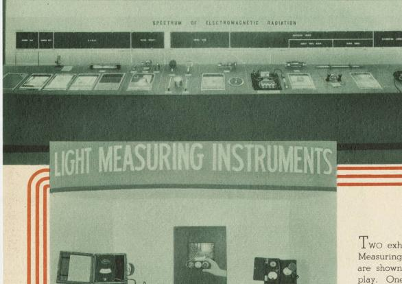
Two exhibits of Light Measuring Instruments are shown in this display. One, the modern photometer, employs a "photronic" cell, a device that turns light directly into electricity. Measuring the electrical
