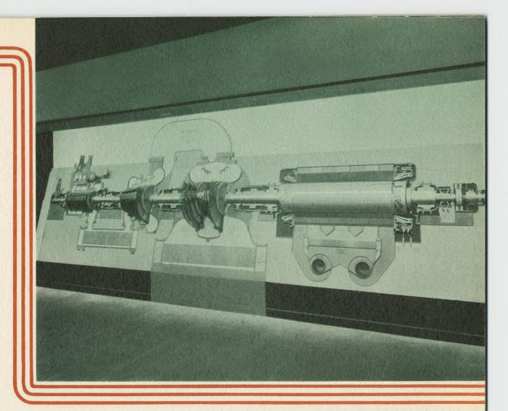
Leaving the third cylinder the steam enters the partial vacuum of the condenser where it returns to the state of water and is carried back to the boilers to begin the cycle over again.
