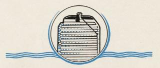
Something that is not generally known is that Pontiac is the only lower priced motor car having a cross flow radiator. This means that the water enters the radiator on the side instead of at the top, which prevents the formation of rust or sludge. It also practically eliminates the evaporation of water or anti-freeze liquid.
