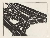
The Pontiac frame is of the K-Y girder type, with greatly increased strength and ruggedness for safety and freedom from road shock. The strong bracing members prevent distortion of the frame, even over the roughest of roads.
