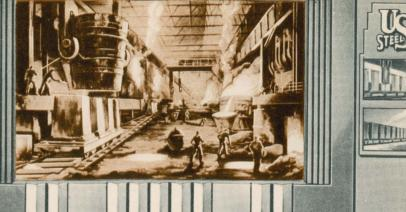
A fiery ten hour process in the open hearth furnace, where the
