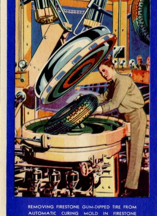
REMOVING FIRESTONE GUM-DIPPED TIRE FROM AUTOMATIC CURING MOLD IN FIRESTONE FACTORY AND EXHIBITION BUILDING.
