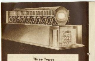
There are three types of electric furnaces: Resistance, Induction, and Arc. They all work on the principle of changing electrical energy into heat energy. In these exhibits, a model of each type of furnace and the principles of its operation are demonstrated
