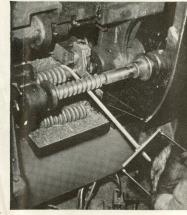
Forming Knee-Action coil spring. A red hot bar of spring steel wraps around the winding arbor, automatically guided to produce the required space between the coils. When the winding is completed, the coil spring drops into the tray below.
