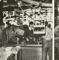
All parts required for assembling Knee-Action units—springs, housings, covers, support arms—arrive at their proper places along the line on overhead conveyors. Skilled workmen rapidly complete finished units.
