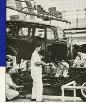
on the Chevrolet chassis. A hoist picks up the body on the Fisher line, swings it through the air to the Chevrolet line, and gently lowers it on the chassis. Workmen tion, and within a few minutes the
