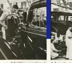
Dozens of finishing operations in rapid-fire order. The radiator, tion—mounting the Fisher Body already assembled, is mounted in place. Hinges and hood catches are installed. Electric wiring is hooked up. Various engine controls are connected. Toeboards, bumpers, hub caps and headlamps guide the body into proper posiare added one by one, and another Chevrolet car is nearly complete. body is securely bolted in place.
