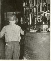
Each coiled spring is heated in an oven to a temperature of 1600 degrees, then it is quenched in oil. The above photograph of the heat treatment shows a workman placing coils in the quenching machine, which holds the coil in correct shape during the operation.
