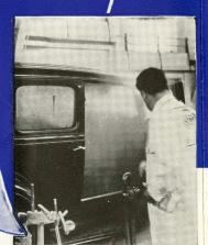
Water for the radiator, fuel for the gasoline tank—then a spray of steam to raise the nap on the upholstery to bring out its sheen. Now a workman starts the engine for the first time. Final inspectors search carefully to see that every operation has been performed perfectly—up to Chevrolet's high standards for dependable service!
