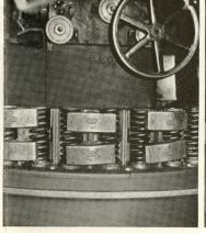
This revolving table is circular, and holds 16 coil springs. After one revolution of the table, one end of each spring has been ground smooth and square. The spring is then reversed to grind the other end.
