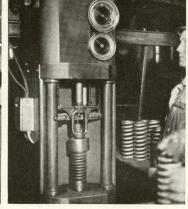
After heat treatment, the coil is compressed to its limit under a load of 3830 pounds, then released under pressure to a height of 8 inches. Large dial gauges enable the operator to check each spring for uniformity, rate and load.
