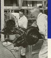
The Knee-Action assemblyshown for the first time in a public exhibit. The 1934 Chevrolet "front axle" is in reality a strong, immovable part of the frame. The big, fully-enclosed Knee-Action units are installed on the ends of the axle—assuring the Chevrolet owner of a far more comfortable ride, shock-proof steering, and a safer ride as well.
