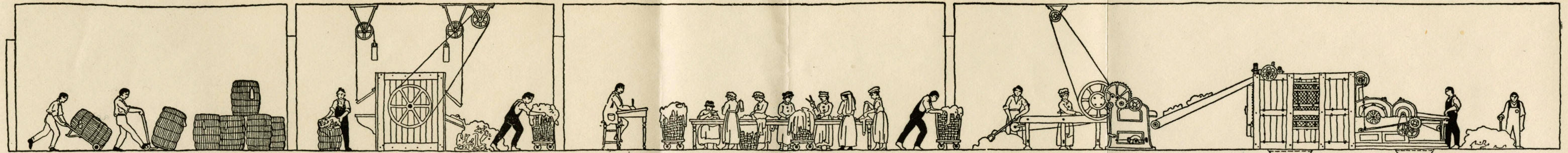
1. The bales of rags arrive at the Mill. 2. The rags are put thru a "Thrasher" which separates them and removes the loose dirt. 3. In the "Rag Sorting Room" the women throw out odd rags, remove all bits of metal and rubber, and cut the rags into strips. 4. The rags are cut into small bits and carried on a travelling belt to a "Duster" which removes any loose dirt remaining, and are dumped thru a trap door in the floor into the "Bleach Boiler."
